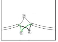
2,Connect the wire of the mirror to the wire of the plug and plug it into the socket
