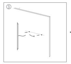
Connect the mirror wires with your main wires and hang the mounting hole to the screw on the wall.
